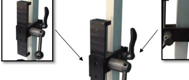
Adjust the height of the force gauge position thanks to the handle
