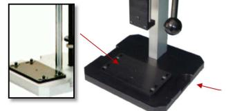
It is recommended that your test stand be secured to a workbench using the mounting holes
